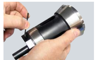
Lock stopper shaft and install
