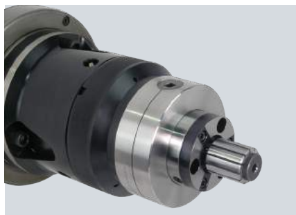
Actuate the power chuck to ensure KEM-MA is locked in position, adjust T.I.R as required.
