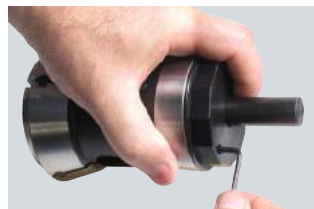
Lock stopper housing in position
